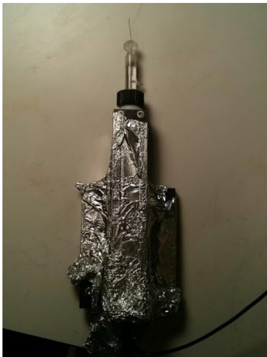
FIGURE 2.5: The pipette holder is rigidly tightened to the preamplifier in the original configuration.
